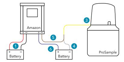
Connect Flow Signal Cable to the Signal-Input port on ProSample.
